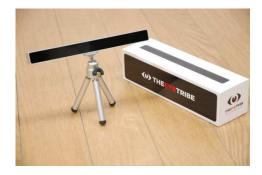
mode with an average accuracy of  $0.5^{\circ}$  and spatial accuracy (RMS) of  $0.1^{\circ}$ . Its operational range varies between 45 and 75 cm. The tool is shown in Figure 3.
